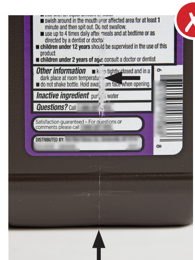
Raised Mold Seam Results in abrasion that makes labels illegible
