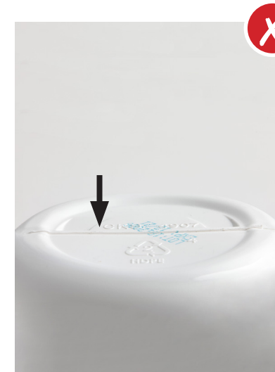
Excess Bottom Flash Results in bottle stability issues, a poor printing surface and a mediocre brand impression
