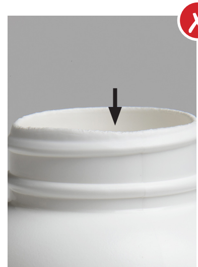
Uneven Sealing Surface Results in poor closure seal and increased risk of product contamination
